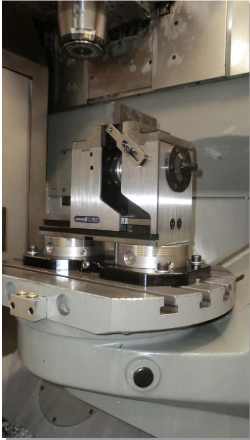
VERO-S NSL plus 200 with clamped KSX 125 – manual vise for 5-axis machining
