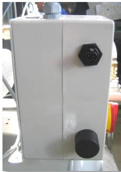
Junction box with potential-free contact and audible warning device
