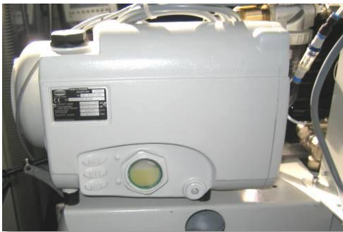
Vacuum pump with sight glass (Oil level)
