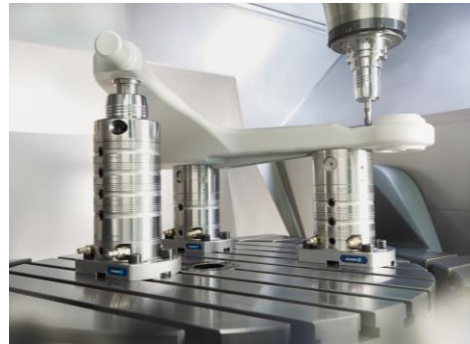
Direct workpiece clamping
