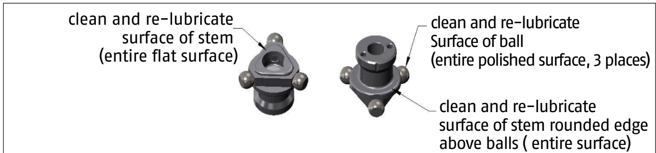
Cleaning and Re-lubricating the Stem
