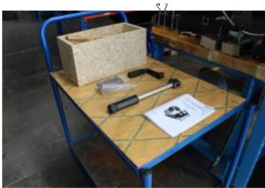
KONTEC KSX incl. Clamping lever, Hand crank and clamping claws
