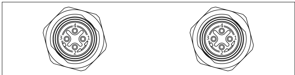
PIN allocation of socket and socket, PROFINET variant
