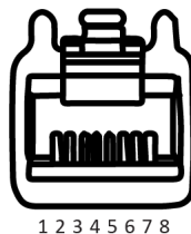
EtherNET-Stecker, RJ45, 8-polig, Buchse
