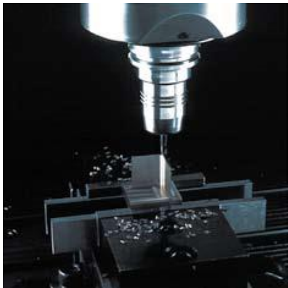
High-speed milling of a copper electrode
