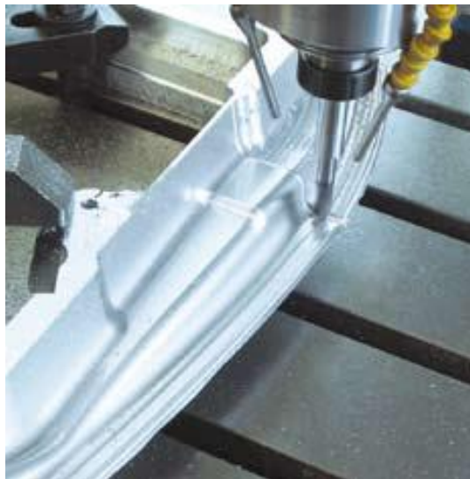
Profile-cutting in finishing of hardened steel with TRIBOS SVL
