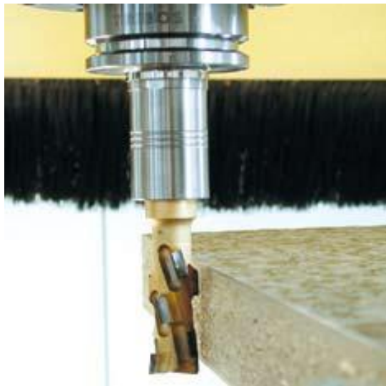
Lateral milling of kitchen countertops with TRIBOS-S (wood working)
